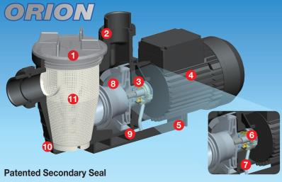
Situated between the pump's wet end and motor, a mechanical seal forms a seal around the motor shaft to prevent water from running out along the motor's shaft. The mechanical seal is the wearing part of any pool pump.
