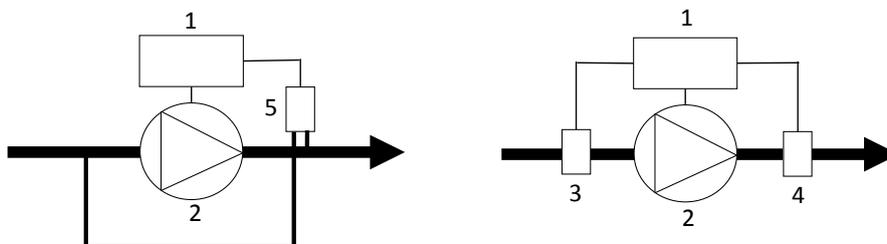
1: Inverter; 2: Pump; 3: Pressure sensor; 4: Pressure sensor; 5: Differential pressure sensor
