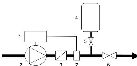
1: Inverter; 2: Pump; 3: Check valve; 4: Pressure vessel; 5: Gate valve; 6: Gate valve; 7: Pressure sensor
