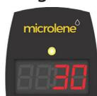
Screen showing 30 days lamp life remaining and amber LED - time to prepare for lamp replacement
