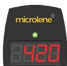
Screen after new lamp inserted successfully showing 420 days lamp life
