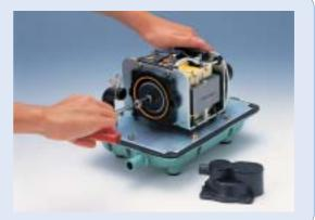
Remove one of the diaphragm mounting blocks from the actuating rod and pull out the other diaphragm mounting block with the rod and finally, separate the diaphragm mounting block and rod.
