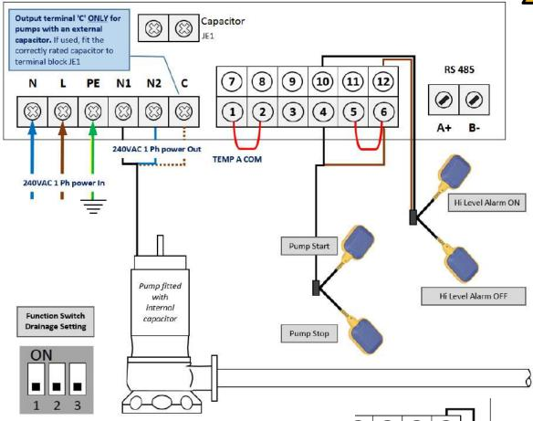
When operating a pump with its own float fitted, tie the float in the upward (permanently on) position.
