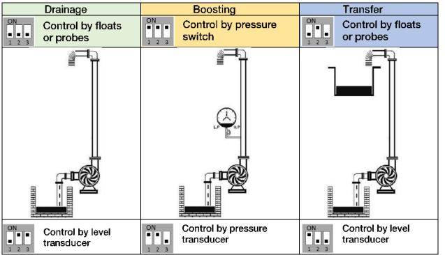
Function switch located upper right-hand side of main board. Cycle power after changing.
