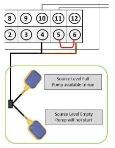
Fitting floats or probes to register the pump inlet source liquid level will achieve the maximum protection against pump dry-running.
