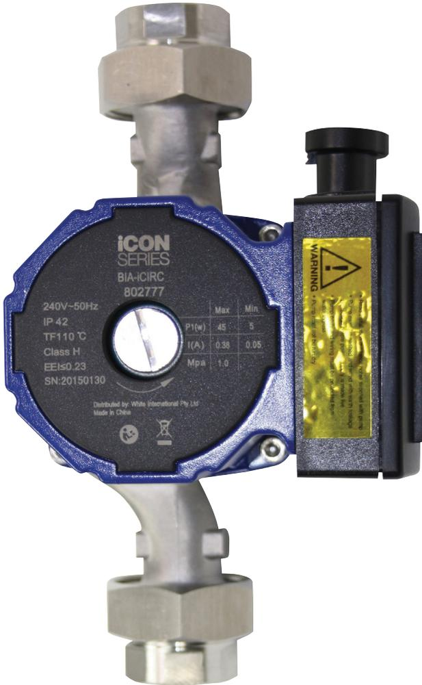
This is a pump used for domestic hot water circulating. The Stainless steel housing makes it suitable for underfloor heating. It is maintenance free and is low in noise. Comes complete with unions. High Efficiency Class A motor. Closed loop VFD motor.
