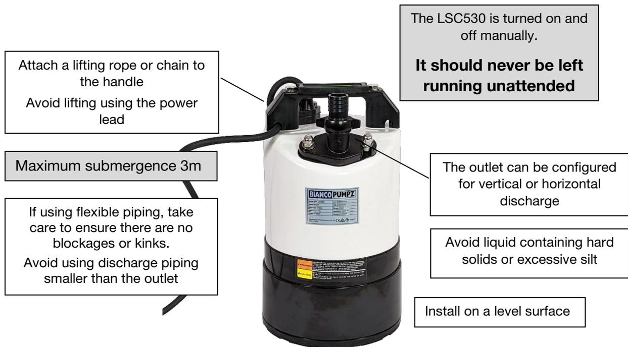
The pump should be connected to (10 amp) power and a residual current device or RCD with a nominal trip current installed in compliance with the requirements of AS/NZ 3000.
