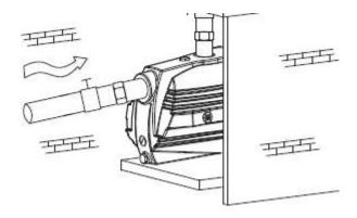
For pump installations, the inlet (or suction) pipe should be as short as possible with the least number or bends. The pump should be installed in a ventilated environment. It could be installed outside, provided the pump is adequately covered from the elements.
