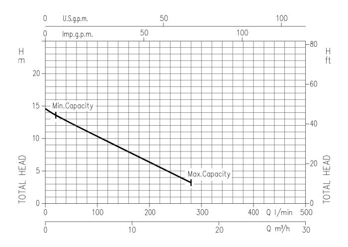
Temperature of water: 20°C Impeller diameter = 120 mm Applicable standard of test: ISO 9906 – Annex A
