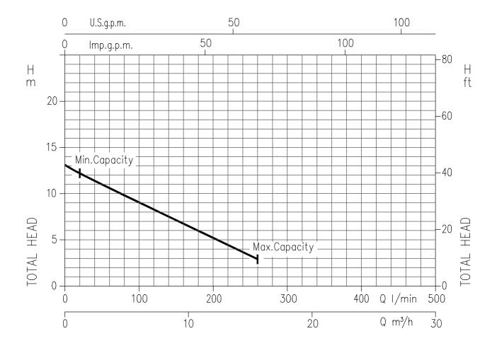
Temperature of water: 20°c Impeller diameter = 112 mm Applicable standard of test: ISO 9906 – Annex A
