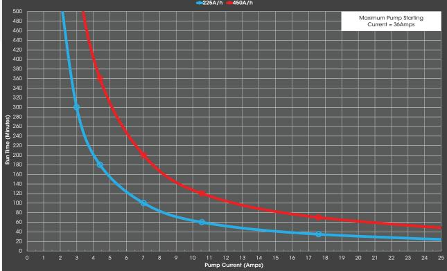
Note: Run time based on new batteries at full battery charge and 25°C. Run time will be reduced with battery age and number of discharge cycles.
