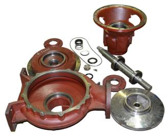
A pump which has become worn in the body or impeller may be repaired by fitting bronze wear rings. These rings, with full instructions for machining the pump parts and fitting rings are obtainable from the nearest Southern Cross Dealer.
